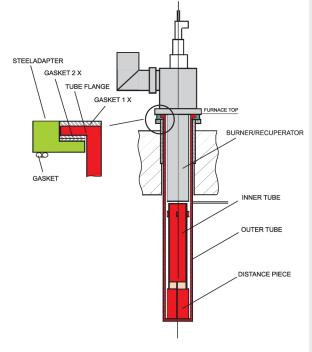
Si/SiC radiant tubes can be used in all heat treatment processes in gas or electrically heated hardening or tempering furnaces and adapt to your existing burners.
